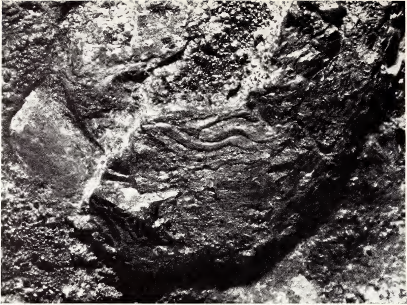
FIG. 13.—34.11. Chinese bronze dagger axe. The macrograph ( \times 10 ) shows traces of a laminated structure in the iron rust which is characteristic of the mineral goethite. This small area of laminated structure occurs about 2 cm. from the end of the bronze blade in an area of rust that was transported and deposited on the bronze surface.
